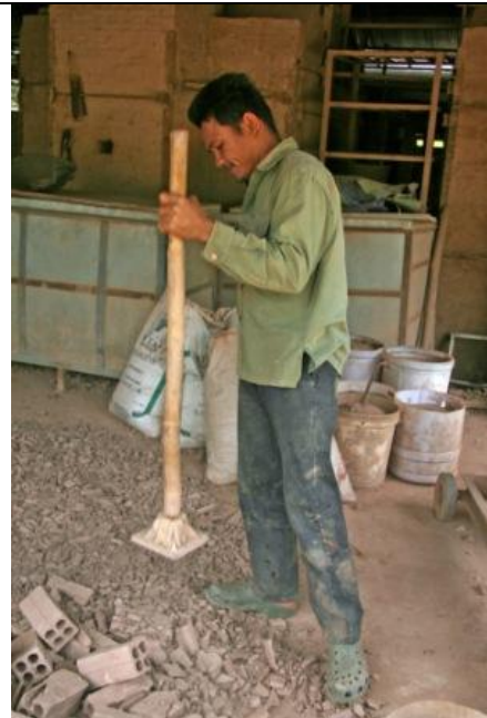
Figure 4.2 Crushing brick with elephant's foot (old method of crushing bricks)
