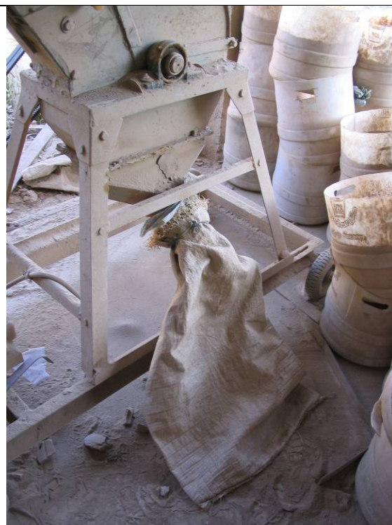
Figure 4.6 Hammer mill discharge with rice sack attached
