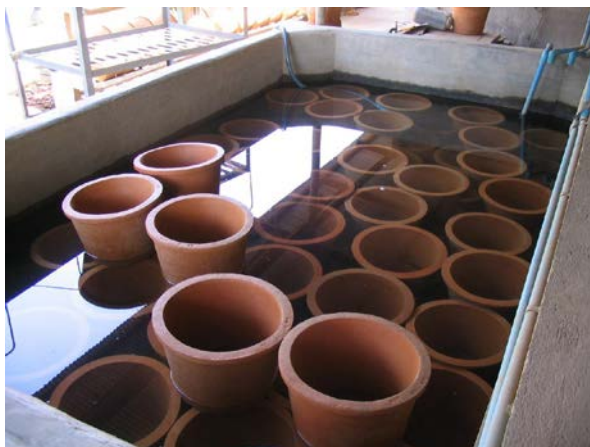
Figure 4.14 Soak bath for flow rate test process
