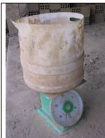
Figure 4.7 Scales for weighing out clay powder from the hammer mill.
