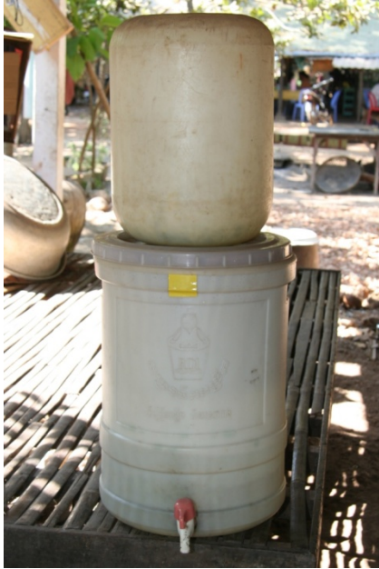
Figure 1.4 Ceramic water filter with additional 20L storage tank attached on top (see also Figure 4.47)
