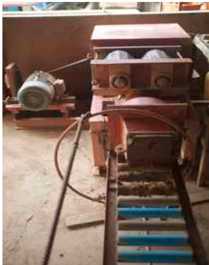
Figure 4.13 Clay pug-mill for forming cubes
