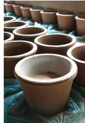
Figure 4.18 Freshly pressed filter element with plastic bowl to hold the shape
