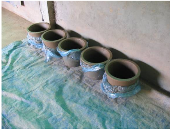
Figure 4.19 Initial drying of filter elements
