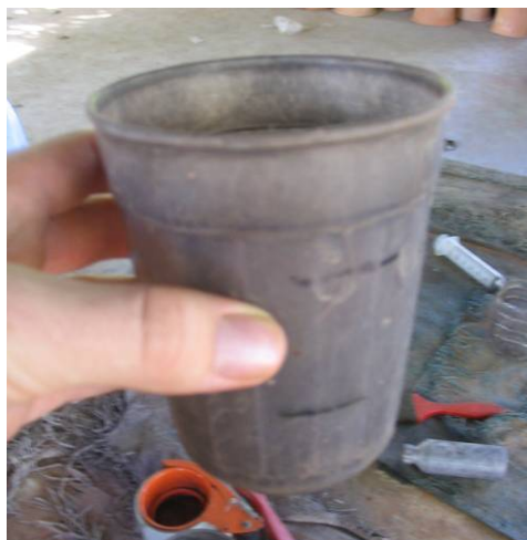
Figure 4.20 Cup for measuring silver nitrate solution (note 2 levels marked)
