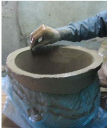
Figure 4.16 Smoothing the edges of newly formed filter element
