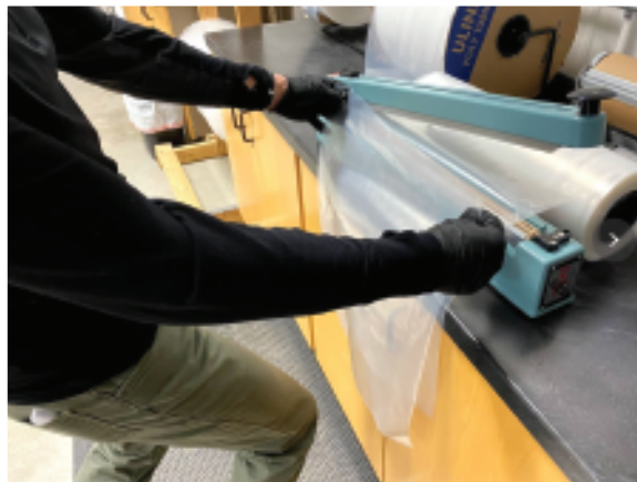
Find a bag that will fit the number of shields you want to ship. We ship in packs of 10 and use a heat sealer to cut and seal the bags.
