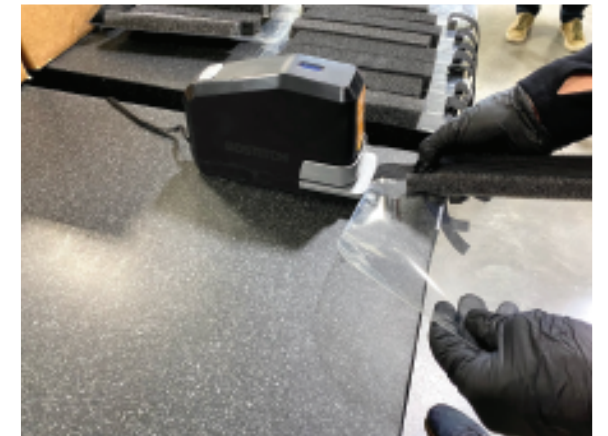
Compress the foam with your thumb to get the elastic to lay flat. Staple the other end of the strap.
