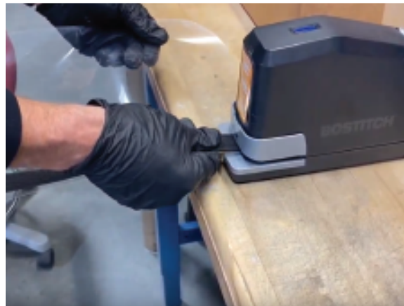
Insert into electric stapler. This should staple about 3/4" from end of strap.
