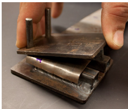
Sheet metal corn sheller forming jig.
